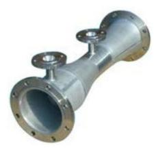
The classical venturi consists of a convergent cone section, cylindrical bore and divergent cone section. While the throat section produces the differential pressure the inlet and outlet cones help in high pressure recovery. This results in lower permanent pressure loss and higher flow capacity than any other differential type flow element of the same size. The outlet cone can be either long (7°) or short (15°) depending upon application.
